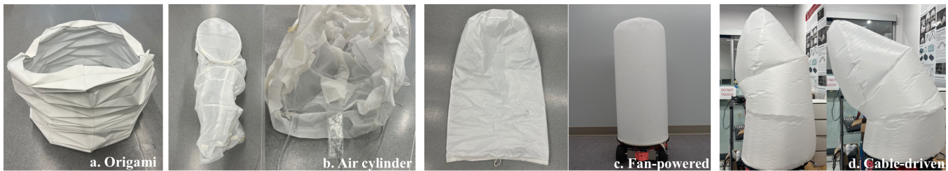
Figure 2: (a) Origami design. (b) Cylinders with valves sewn in along the sides of the bladder. (c) Fan-powered tubular bladder. (d) Experimenting with cable-driven motions on lipstick-style bladder.
