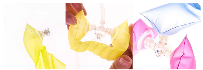
Figure 6: (a) Oral inflation valves with plug, (b) T-shaped connector joining two ends of the same module, (c) three modules connected with a cross-shaped connector.
