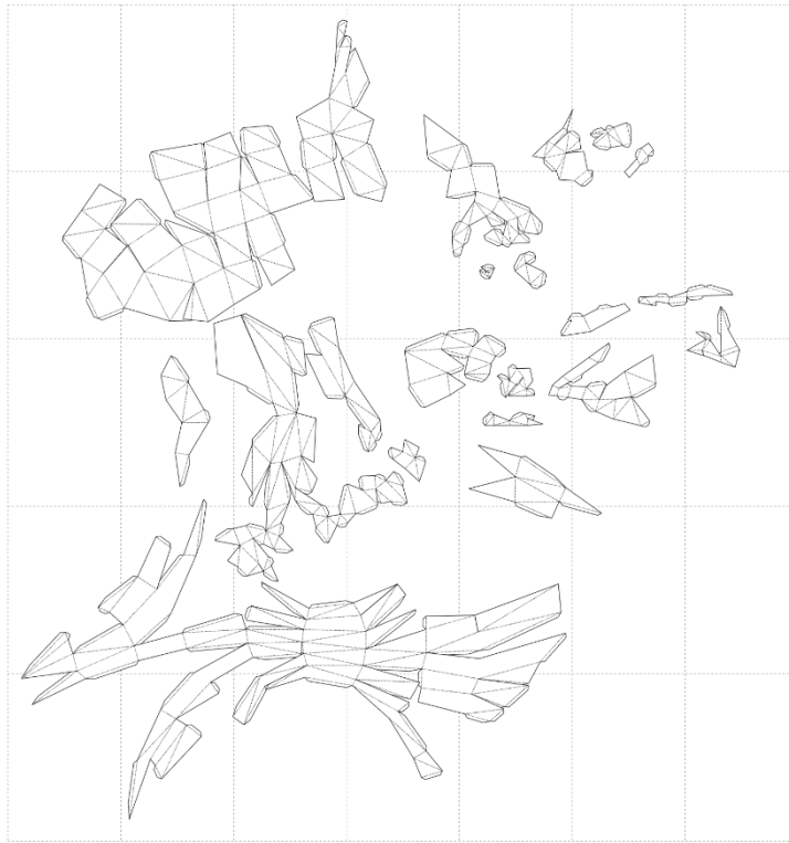
Figure 2: A 3D design unfolded into multiple 2D patterns using Pepakura software.
