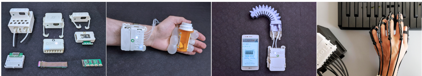
Figure 1: (a) The FlowIO platform with all modules. (b, c, d) Three application scenarios utilizing the small, medium, and large pump modules for (b) wearable, (c) desktop, and (d) hybrid wearable & desktop applications, respectively.
